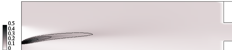
Figure 3 Contour plot of mean mixture fraction in the symmetry plane, of the IFRF furnace. Contour lines denote values of 0.1 to 0.5.
